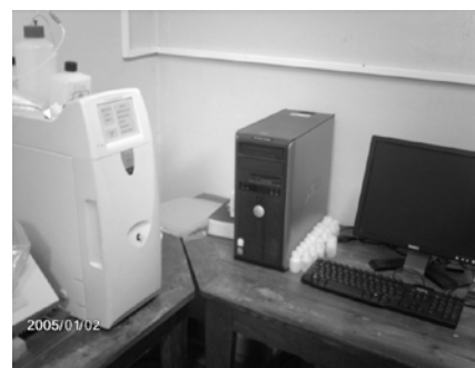
Fig. 2. Ion chromatograph, type Dionex IC1000 connected to a computer
